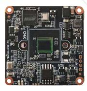
The HM50C01 is a cost-effective 5MP surveillance network camera module designed for both indoor and outdoor use. It features a 1/2.8" Sony IMX335 STARVIS sensor and is powered by the GOKE GK7205V300 SoC, equipped with 1Gb of RAM. It support network video and analog video synchronous output. In terms of extended I/O capabilities, it supports dual light source illumination, as well as microphone and speaker connections, enabling two-way audio and additional interfaces.
