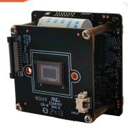
The IM80A01 is a high-performance 8MP surveillance network camera module designed for both indoor and outdoor use. It features a 1/2.8" Sony IMX415 STARVIS sensor and is powered by the Hisilicon 3519DV500 Ai SoC, it integrated with efficient neural network inference engine, with a maximum computing power of 2.5 TOPS. In terms of extended I/O capabilities, it supports dual light source illumination, as well as microphone and speaker connections, enabling two-way audio and additional interfaces.
