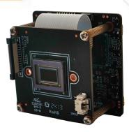
The IM80B01 is a high-performance 8MP surveillance network camera module designed for both indoor and outdoor use. It features a 1/1.8" Sony IMX678 STARVIS sensor and is powered by the Hisilicon 3519DV500 Ai SoC, it integrated with efficient neural network inference engine, with a maximum computing power of 2.5 TOPS. In terms of extended I/O capabilities, it supports dual light source illumination, as well as microphone and speaker connections, enabling two-way audio and additional interfaces.
