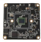
The IM50Q01 is a cost-effective 5MP surveillance network camera module designed for both indoor and outdoor use. It features a 1/2.8" Sony IMX335 STARVIS sensor and is powered by the Sigmastar SSC377QE SoC, equipped with 1Gb of RAM. In terms of extended I/O capabilities, it supports dual light source illumination, as well as microphone and speaker connections, enabling two-way audio and additional interfaces.
