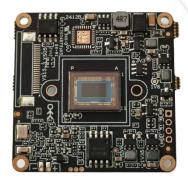
The IM20A03EU is a cost-effective 2MP surveillance network camera module designed for both indoor and outdoor use. It features a 1/2.8" Sony IMX307 STARVIS sensor and is powered by the GOKE GK7205V300 SoC, equipped with 1Gb of RAM. In terms of extended I/O capabilities, it supports dual light source illumination, as well as microphone and speaker connections, supports external sound post interfaces and additional interfaces.
