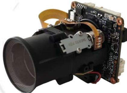
The IM20A01W-4X is a cost-effective 2MP surveillance network camera module designed for both indoor and outdoor use. It features a 1/2.8" Sony IMX307 STARVIS sensor and is powered by the GOKE GK7205V200 SoC, equipped with 512Mb of RAM. It Supports 2.4G WiFi and RJ45 Network Connectivity. In terms of extended I/O capabilities, it supports dual light source illumination, as well as microphone and speaker connections, enabling two-way audio and additional interfaces.
