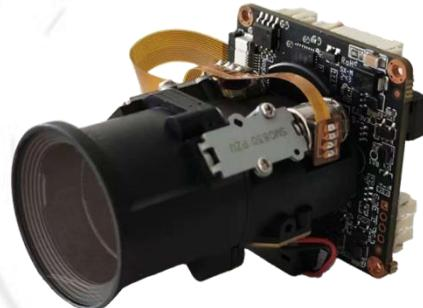
The IM50A01W-4X is a cost-effective 5MP surveillance network camera module designed for both indoor and outdoor use. It features a 1/2.8" Sony IMX335 STARVIS sensor and is powered by the GOKE GK7205V300 SoC, equipped with 1Gb of RAM. It Supports 2.4G WiFi and RJ45 Network Connectivity. In terms of extended I/O capabilities, it supports dual light source illumination, as well as microphone and speaker connections, enabling two-way audio and additional interfaces.
