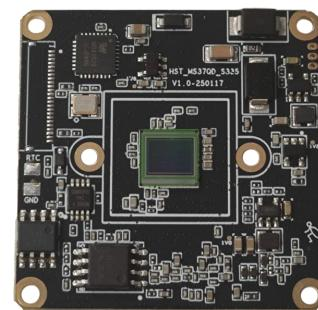
The IM50Q01 is a cost-effective 5MP surveillance network camera module designed for both indoor and outdoor use. It features a 1/2.8" Sony IMX335 STARVIS sensor and is powered by the Sigmaster SSC377QE SoC, equipped with 2Gb of RAM. In terms of extended I/O capabilities, it supports dual light source illumination, as well as microphone and speaker connections, enabling two-way audio and additional interfaces.
